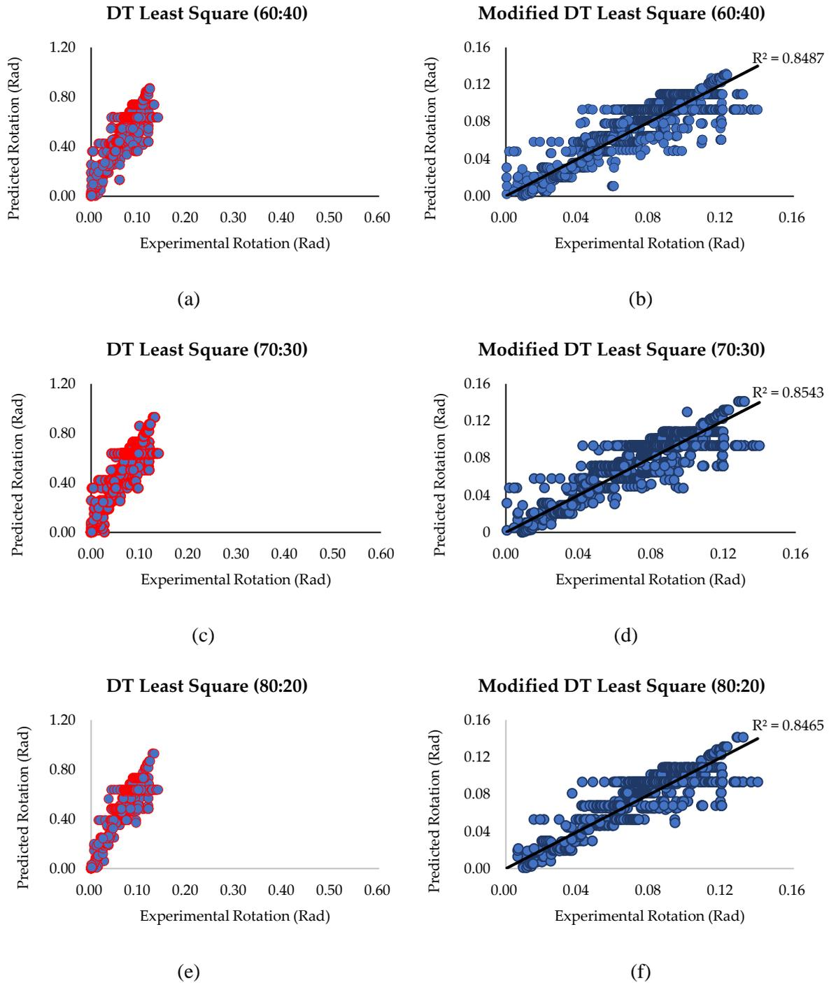
**Figure 9.** Comparison of rotation for DT Least Square and experimental.
