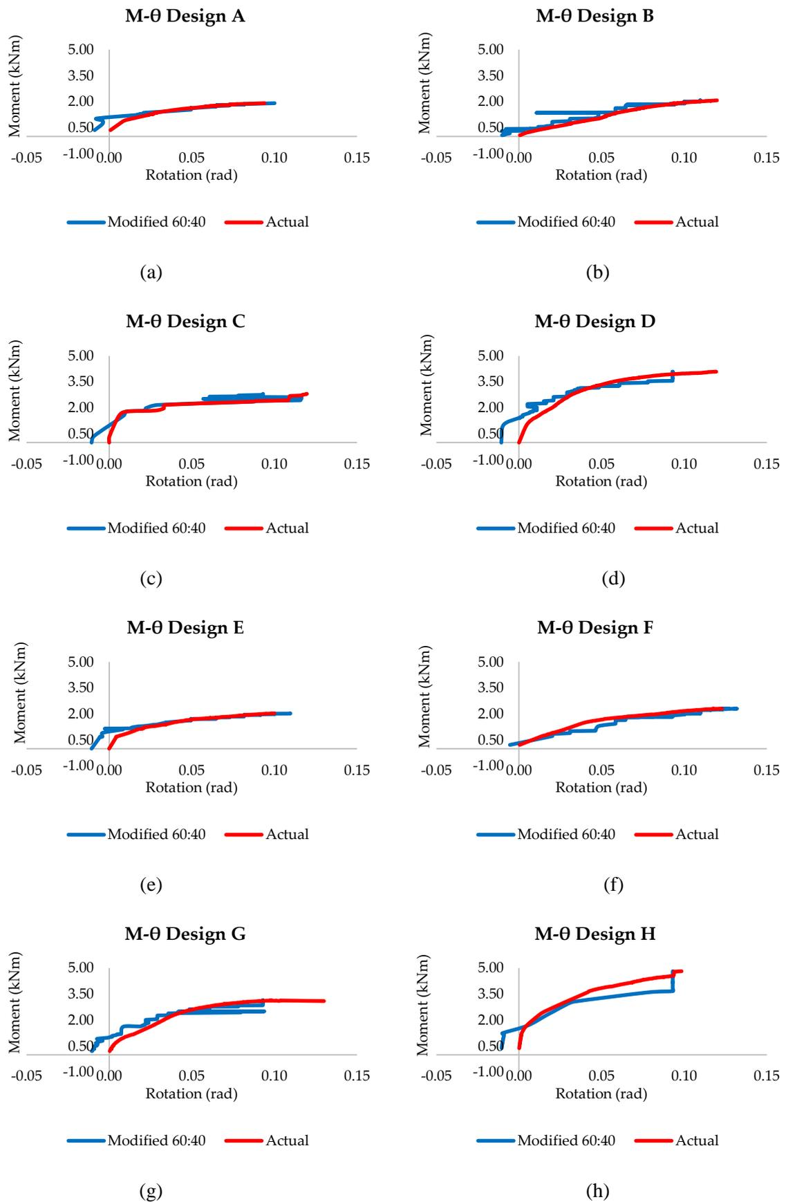
**Figure 10.** M-θ characteristics for different designs of boltless steel connections
