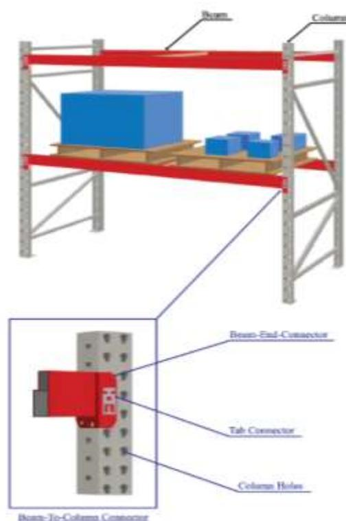
**Figure 1.** Typical steel pallet racking system.
