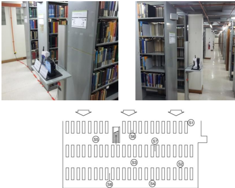
Figure 3: Positioning of YESAIR and YESDUST devices that measure IAQ in the book shelf area at spot S2, while S1 – S9 are grab sampling spots for luxmeter and sound level meter.
