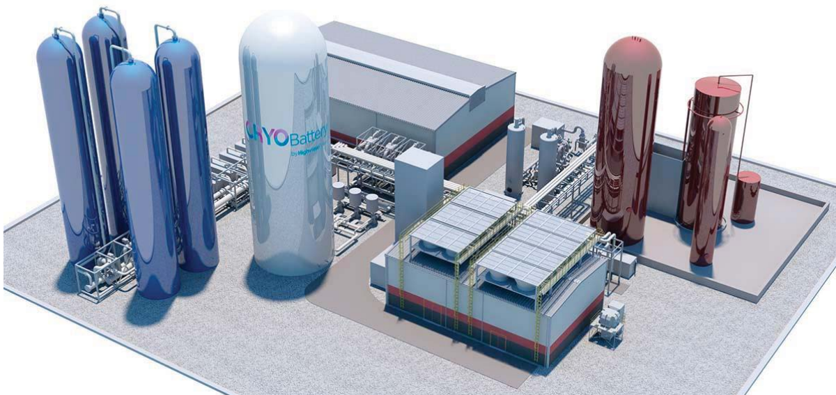
Figure 3. Liquid Air Energy Storage design called CRYOBattery (Sumitomo SHI FW, 2025)
